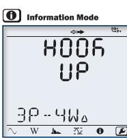
Hook up, voltage and current ratios and aggregation period can be configured from the front panel of the PEL 103.
