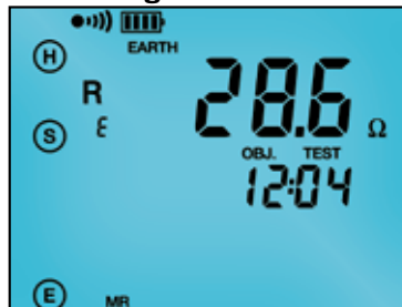
Memory Recall displays test results stored at a specific memory location.
