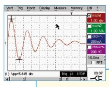
Many complex functions are editable, including simulation of a trace on the basis of its mathematical equation and therefore modelling of an expected result.
